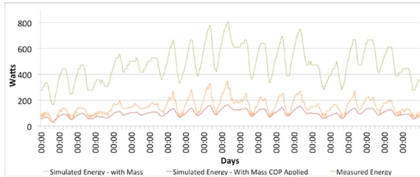
Figure 11: With-mass measured and simulated energy use
