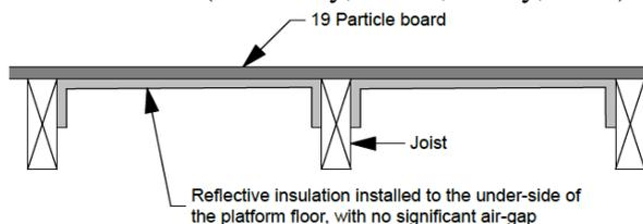
Figure 1: Diagram of reflective subfloor insulation installation
