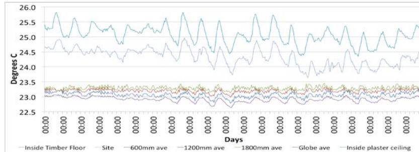
Figure 7: Test cell room measured temperatures
