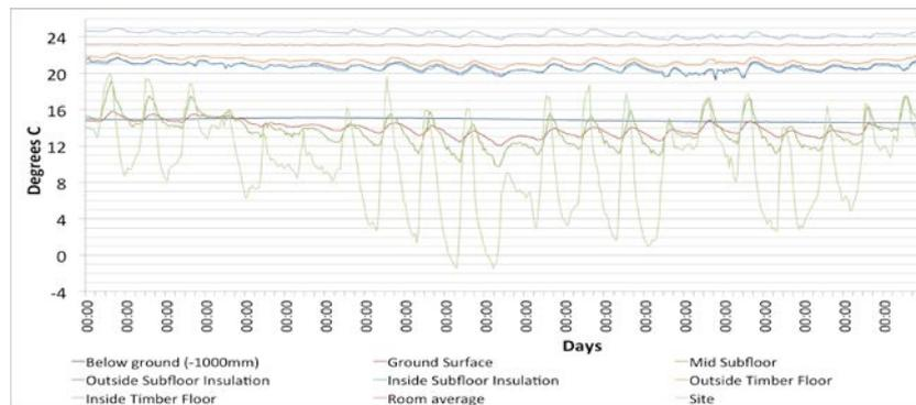
Figure 2: Continuously heated subfloor temperatures
