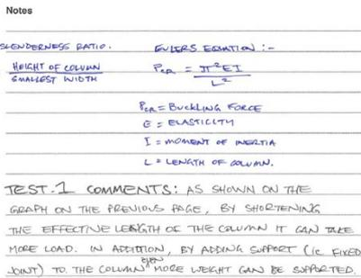
Figure 9: Part of a student's record of the week 3 columns and buckling experiment
