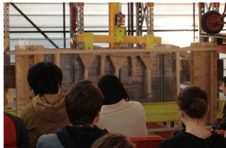
*Figure 2: Week 10 – Trusses that have been designed and manufactured by students are tested for deflection and failure*
