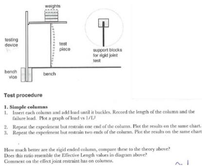
Figure 7: A Week 3 workshop task on columns and buckling
