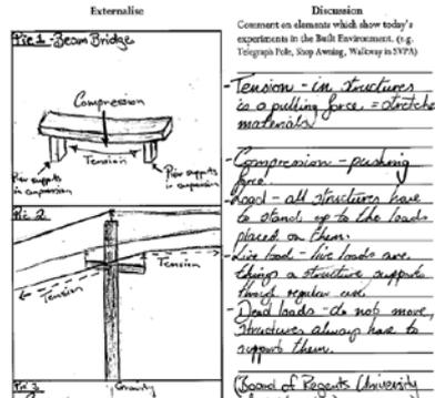
Figure 12: Part of a student's record of the week 3 columns and buckling experiment
